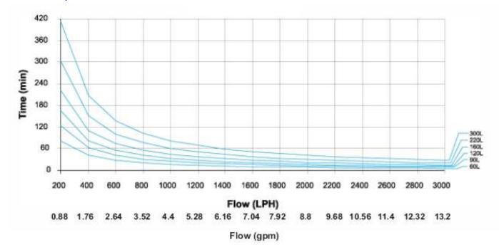
The time that the fertilizer in either fluid or solid state is supplied into the irrigation network depends on the solubility and the quantity of the fertilizer, as well as the flow rate of water through the fertilizer tank.
